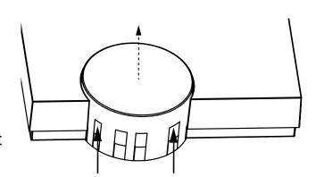
• Press and hold the emergency button (D), while plugging in the power supply cable again, then release.
